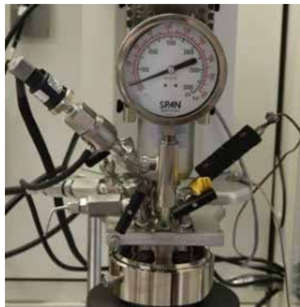
Lab autoclave for hydrogenation tests on plastic waste and model mixtures.
