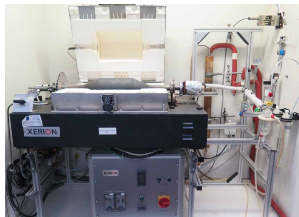
The “pool-in-loop” test facility: a rotary kiln reactor.
